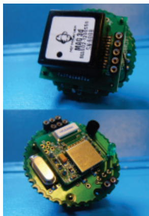
Fig. 1. Electronic sensing core: (up sensing unit, down wireless trasmission board.
