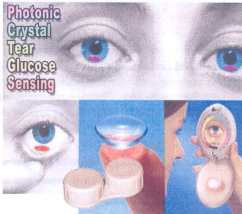
FIGURE 13.1: Photonic crystal glucose sensing material for determining tear fluid glucose concentrations. The sensing material is embedded within a contact lens or ocular insert. The color diffracted changes with the tear fluid glucose concentration. A mirrored compact-like device illuminates the sensor with white light. The sensor color is determined by viewing the reflected (diffracted) light and compared to a color wheel calibrated in blood glucose concentration.
