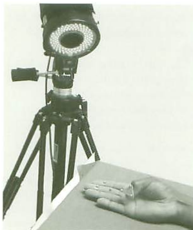
Figure 2. Motion analyses of functional opposition of the thumb using VICON motion capture system
