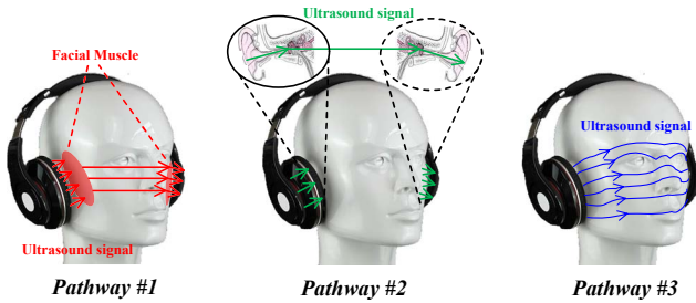
Figure 3: Three possible pathways of ultrasound signal propagation
