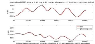
The WiiMoCap system was validated with the data recorded simultaneously from a six camera Impulse system from Phasespace Inc. The Impulse camera system streamed data at 120 Hz. Each camera has a resolution of 3,600 x 3,600 pixels, and a 60 degree field of view.
