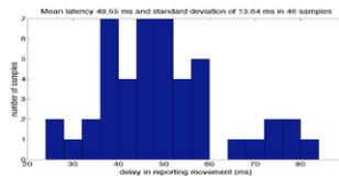
The acquisition delay or latency in a Wiimote includes detection and transmission delays. The mean latency in acquisition of the Wiimote was 49.6 ms (standard deviation 13.6 ms).
