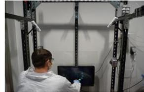
Calibration is the process of converting raw position coordinates reported by a Wiimote into workspace coordinates. Calibration is performed at the beginning of a training session, it is easy to perform and takes less than one minute.
