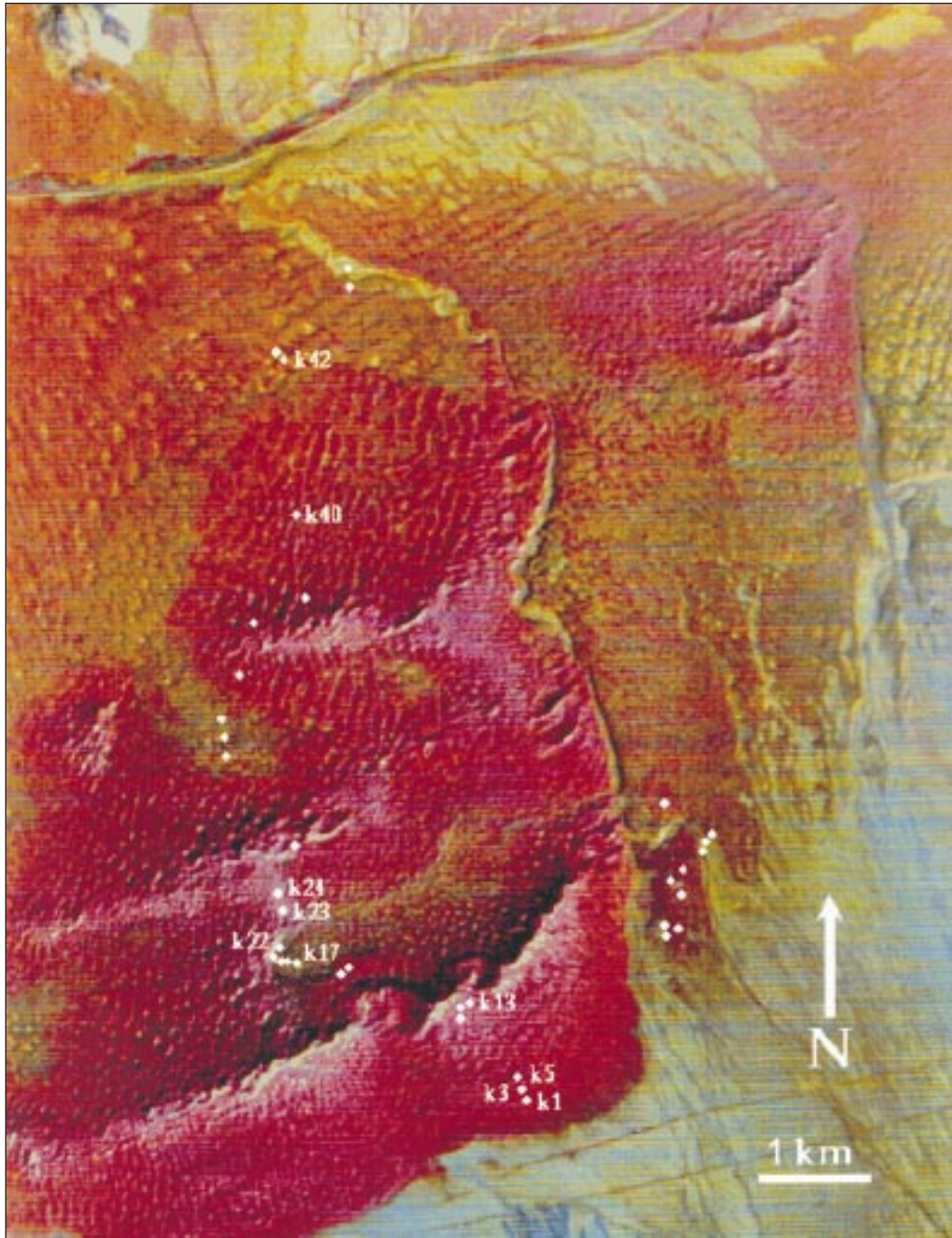
Figure 4. Decorrelation stretch image of the 1984 thermal infrared multispectral scanner (TIMS) data with bands 5 (10.7 \mu\text{m} ), 3 (9.2 \mu\text{m} ), and 1 (8.4 \mu\text{m} ) in red, green, and blue, respectively (see Barbera [1989] for a description of the data). Sand sample sites are shown as white diamonds; numbered samples were used for petrographic analysis. The color changes in the image indicate mineralogic variations, whereas brightness differences show surface temperature changes (see text). Close examination reveals a horizontal “venetian blind” striping that is caused by microphonic noise present in the raw data. This noise is exaggerated upon data transformation using techniques such as the decorrelation stretch and linear retrieval. Together with the limited areal coverage of the surrounding alluvial surfaces, this prompted new TIMS data to be collected in 1995 (Fig. 8).
