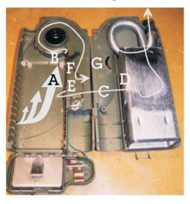
make sense — when the clamshell is folded back together, a little hole in the charcoal box fits (D) snugly up against a black rubber grommet (E) on the fan outflow box. If you also look at (F) you'll see a little piece of black plastic, which has a tiny black nubbin that sticks out through a curved hole in the case (G), and allows you to adjust the heat (see Figure 7 for an outside view of it).
