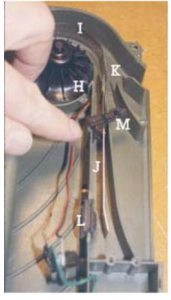
high-low lever — by adjusting this up or down, you can increase or decrease the air going into the charcoal box, and increase or decrease the heat. Of course if you turn it up full blast, it won't run as long on a charcoal charge, but then even at full blast 200 Watts it lasts for 6 hours (20 hours at 50 Watts on low), and the charcoal charges are light, so you can easily carry a few extras.
