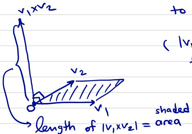
Right-hand rule (to decide direction of  $v_1 \times v_2$ )
