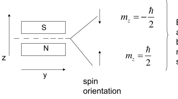
Beam of Ag atoms split by inhomogeneous magnetic field – 2 wellseparated peaks seen
