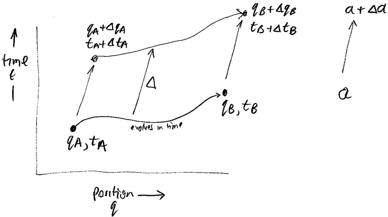
compute change in action  $\int_{t_A}^{t_B} L dt$  under  $\Delta$
