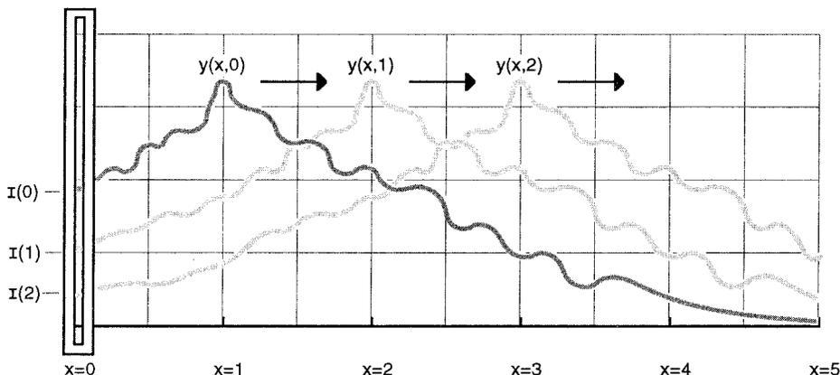
Figure 4. Retarded solution of one dimensional wave equation.
