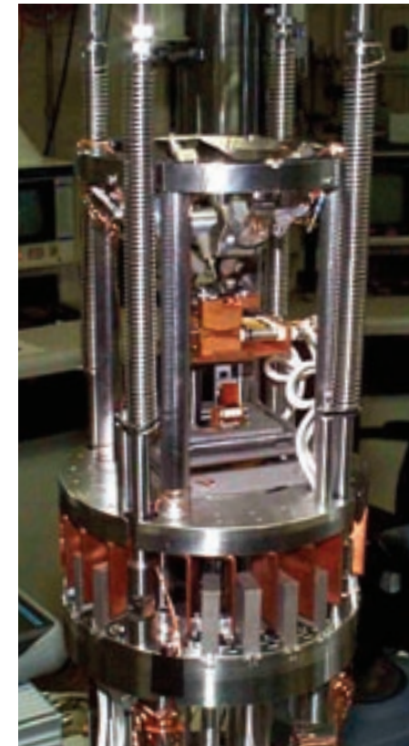
The nanoworkbench developed by John T. Yates, Jr., and coworkers is used by nanoscale investigators. Its four-probe scanning tunneling microscope (STM) moves a tiny metal probe across a specimen's surface.
