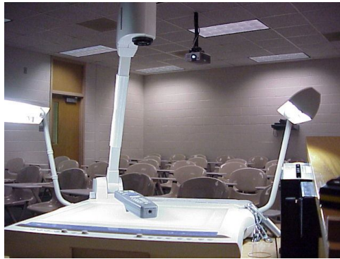
Fig. 9.10 Sony's DC-13 document camera connected to the ceiling-mounted projector
