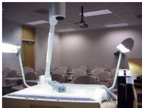
Fig. 10.11 Sony's DC-13 document camera connected to the ceiling-mounted projector
