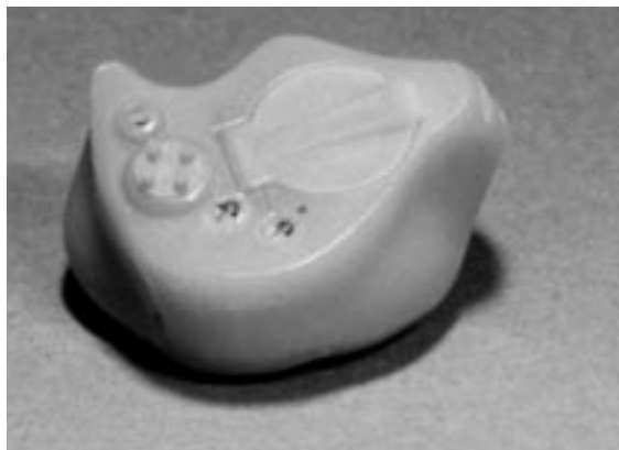
Figure 6 This shows an in-the-ear hearing aid.
