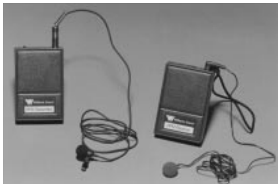
Figure 9 Assistive listening device to overcome noise and distance problems
