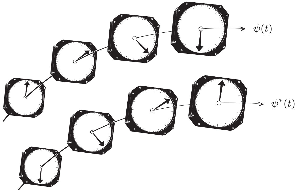
Figure 2: Conjugating the wave function has the effect of ‘flipping’ the arrow about the real axis of the dial. The resulting conjugate wave function corresponds to a dial that spins in the reverse direction.
