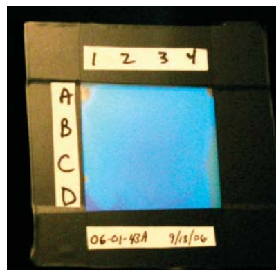
Figure 1. 3 cm \times 3 cm TGCCA fabricated between glass plates by using a 100 \mu m thick polyester spacer to separate the TGCCA from the adhesive used to seal the edges of the glass plates. The cell was divided into 16 9 mm square regions (A1–D4) that were analyzed via UV–vis transmission spectroscopy by using a 5 mm diameter aperture.
