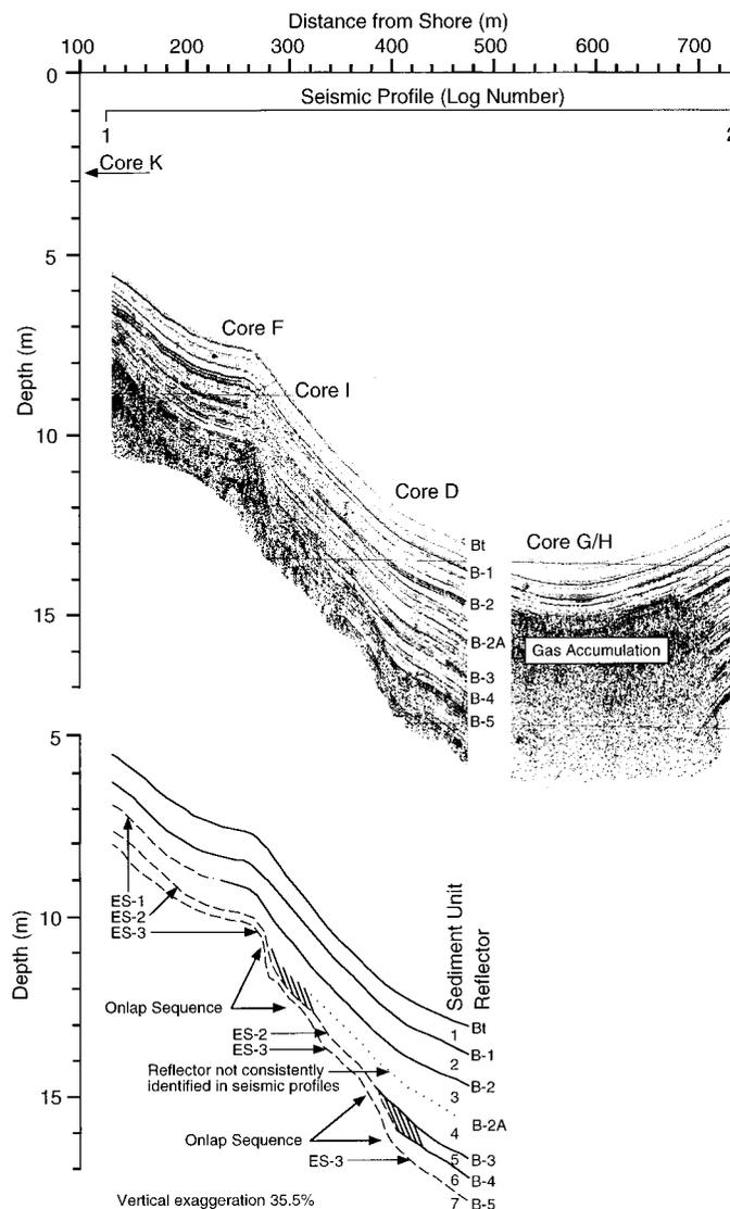
FIG. 3. Seismic profile 1-2 from the southern basin of Birch Lake, filtered between 3 and 7 kHz, illustrates the acoustic stratigraphy along the transect of cores K-G/H. Note the two sets of onlap sedimentary sequences formed during lake-level transgressions and erosion surfaces 1–3 highlighted by the illustration in the lower part of the figure. The zones of gas accumulation are limited to the center of the lake and to the sill separating the two basins.
