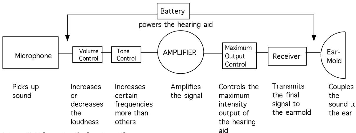
Figure 5 **Schematic of a hearing aid.**
